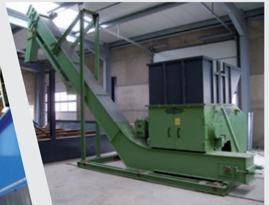
Shredder with discharging trough chain conveyor
