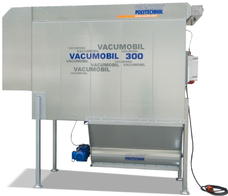
Fig. above: Vacumobil VZ 300 with vibrations cleaning and rotary valve
