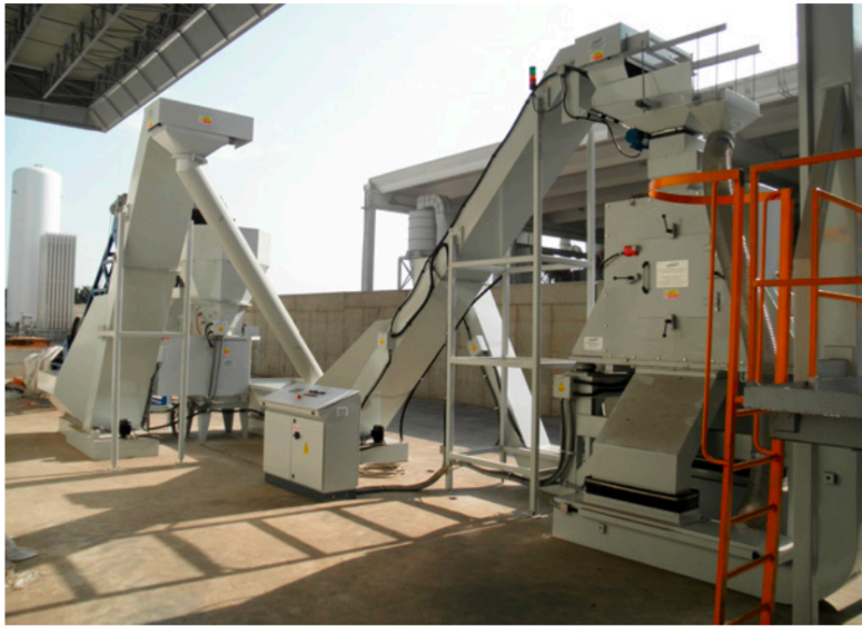
Crushing and spinning system. Capacity: 3 ton/h for aluminium swarf
