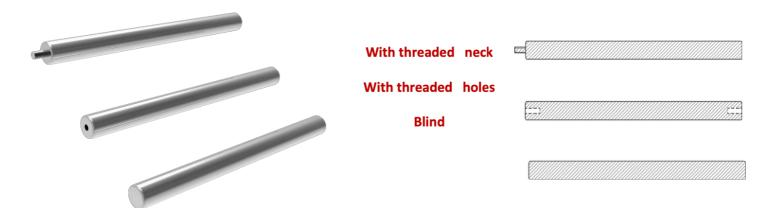
We manufacture them according to each project requirements, depending on the product to be filtered, the particle size of the material, the stream flow and the available space. They are mainly made in 25 mm or 32 mm diameter. The length will depend on the application, generally between a range of 100 mm to 1800 mm.
